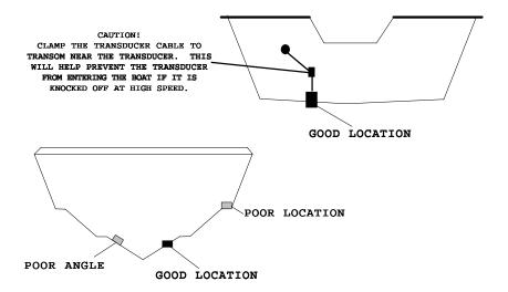
4. Hold the transducer and bracket assembly against the transom. The transducer should be roughly parallel to the ground. The bottom of the transducer bracket should be in line with the bottom of the hull. Don't let the bracket extend below the hull! Mark the center of the slots for the mounting holes. Drill two 5/32" holes in the marked locations for the #10 screws supplied with the transducer.
